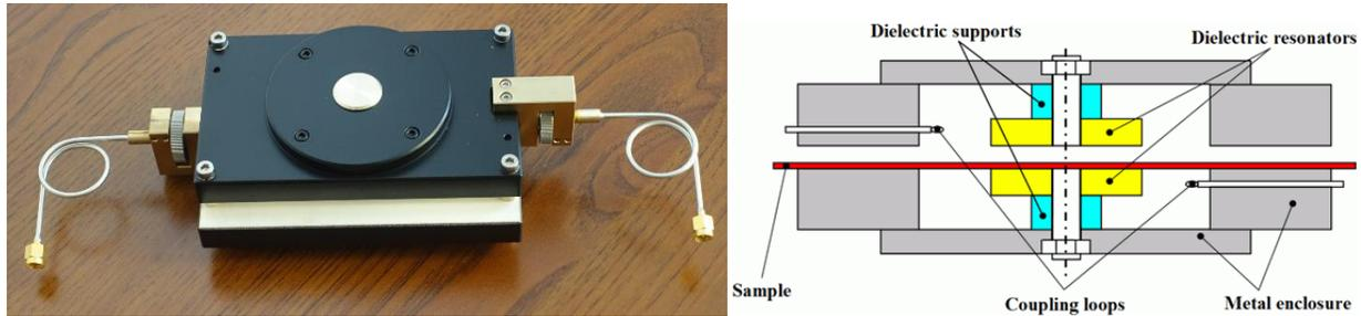
Fig. 1: Example SPDR and its internal construction after [1][2][3].
