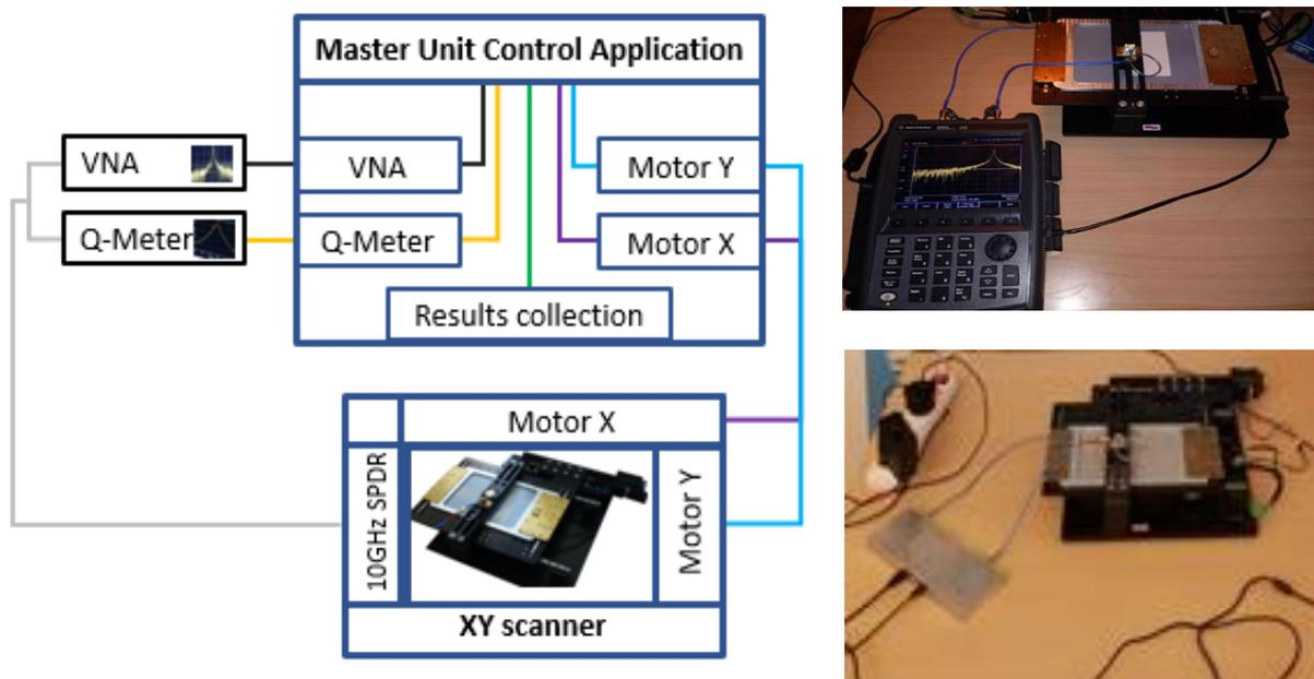
Fig. 5: Block diagramme of the 2D SPDR scanning setup (left) and validated connections of the scanner to KEYSIGHT FieldFox (upper right) and QWED Q-Meter (lower right).
