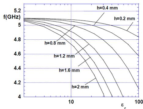
Fig. 3: Resonant frequency ( $f$ ) of an example (nominally) 5 GHz SPDR loaded with a SUT of height  $h$  and relative permittivity  $\epsilon_r$ .
