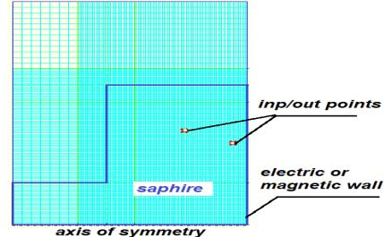
Fig. 2. Considered 2D model of the resonator in BoR FDTD software [3].
