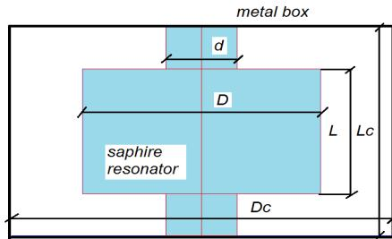
Fig. 1. The considered dielectric resonator after [1]. Sapphire in-plane and out-of-plane relative permittivities are 11.3532 and 9.2747, respectively;  $D_c = 80$  mm,  $L_c = 50$  mm,  $D = 49.9894$  mm,  $L = 30.008$  mm,  $d = 15$  mm.
