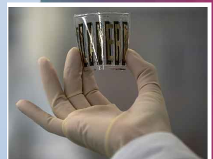
LAYER® OPV module by inkjet printing
