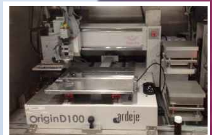
Inkjet printer in the Dracula Technologies' LAYER® LINE
